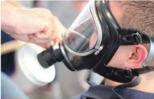
Figure 11.5: Full face mask with Rd 40mm (CEN) test adapter and P3 filter
