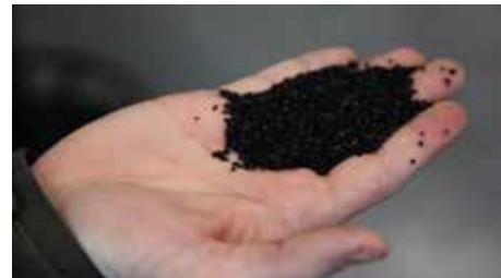
Figure 5.1: Granules of activated carbon
