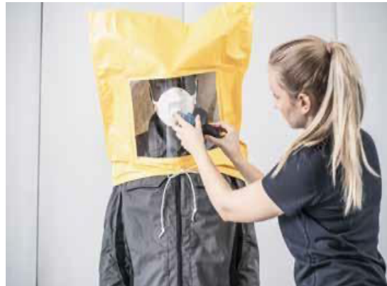
Figure 11.2: Qualitative face-fit test
