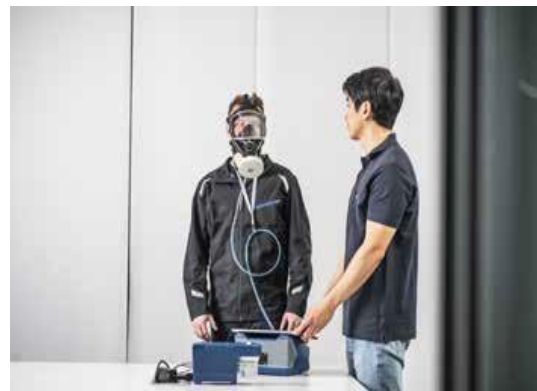
Figure 11.3: Quantitative face-fit test
